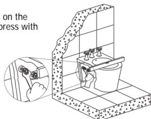
6 Measure the siphon with 200mm (7 7/8") from the wall. Set the caulk ring in the 40mm (1 9/16") knee. Next set up the siphon.
