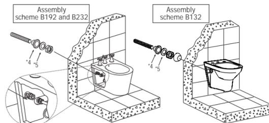
5 Check if the bidet is on the right level and compress with an appropriate tool.
