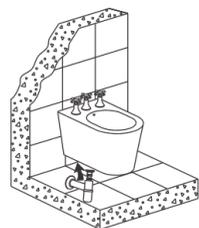
7 For a perfect finishing, apply white cement on the contact region on the wall.
