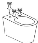
3 Approach the bidet on the wall and connect the flexible.
